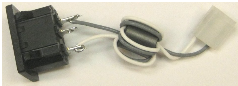
Figure 68 – Supplemental CM Choke (4T on Fair-Rite 5943000201).
